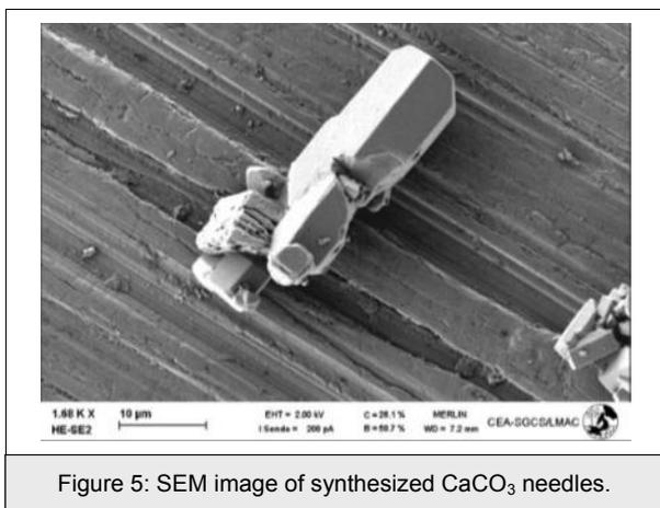
Figure 5: SEM image of synthesized CaCO<sub>3</sub> needles.
