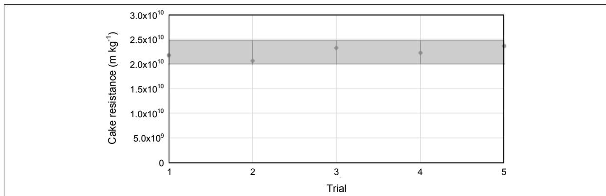
Figure 3: Exemplar repeatability measurement distribution for the Filtration Performance Test.
