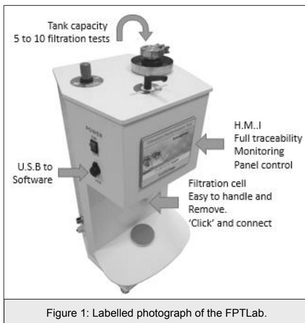
Figure 1: Labelled photograph of the FPTLab.
