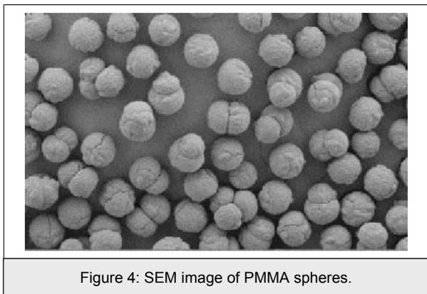
Figure 4: SEM image of PMMA spheres.
